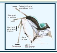
The **tether** is located on the upper part of the back of the car seat.
