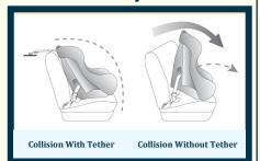
If the vehicle manufacturer does not state a weight limit, do not use the tether if the weight of the child + the car seat combined is greater than 65 pounds.
