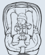
Car safety seat with a small cloth between crotch strap and infant, retainer clip positioned at the midpoint of the infant's chest, and blanket rolls on both sides of the infant.
