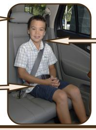
Shoulder belt is placed across the center of the chest and shoulder and in contact with the child's shoulder.
