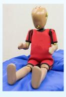
DEPARTMENT OF TRANSPORTATION National Highway Traffic Safety Administration 49 CFR Part 572 Docket No. NHTSA-2020-0088 RIN 2127-AL04 Anthropomorphic Test Devices; Q3s 3-Year-Old Child Side Impact Test Dummy; Incorporation by Reference
